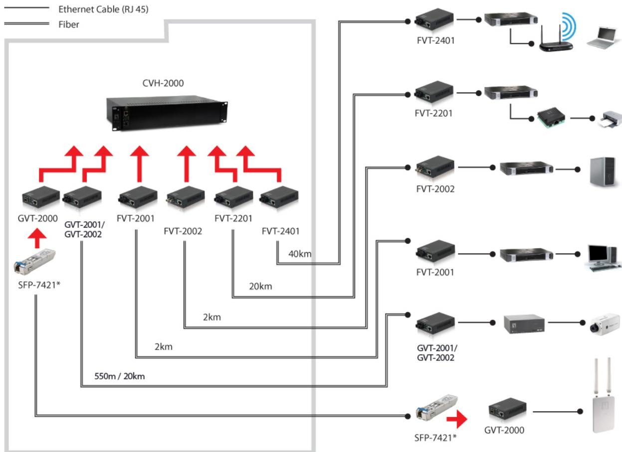
\*In above example diagram, converter modules at local and remote ends should be paired for proper connectivity, and the distance mainly depends on cable and transceiver selection accordingly.
