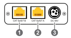
① CAT 5e/6/7 B Port: Connect to a compatible unit with a single Cat.5e/6/7 cable for bypassed transmission of all data signals. PoE/PoH can also be supplied to compatible PD devices if the feature has been enabled via the appropriate front panel switch.
